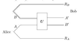
The double lines indicate the very large systems B and B', and single lines the smaller systems A and A'. Because the radiated qubits are random, we can determine whether  $R_AB'$  decouples using the decoupling inequality, which for this case becomes
