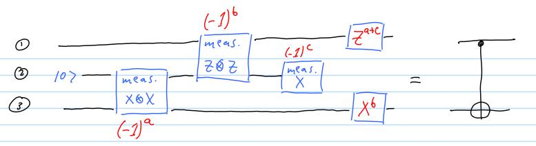
Here  $(-1)^q$  denotes the outcome of meas of  $X \otimes X$ , etc., and  $Z^{a+c}$  means apply 2 conditioned on parity of outcomes of  $X \otimes X$  and X meas.
