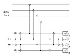
The four-qubit cat state is encoded with four qubit preparations and three CNOT gates, the ancilla interacts with the data block via four CNOT gates, the ancilla is decoded with three CNOTs, and then all four ancilla qubits are measured as shown.
