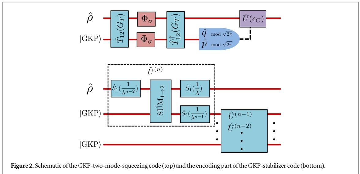
Figure 2. Schematic of the GKP-two-mode-squeezing code (top) and the encoding part of the GKP-stabilizer code (bottom).
