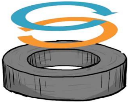
Persistent current in a superconducting circuit
